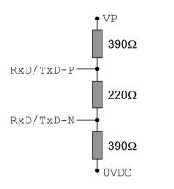
If the device is at the end of the network, use a Profibus connector with terminating resistor.
