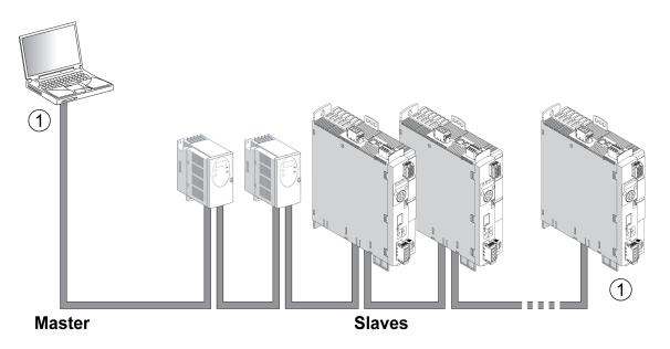
1 Both ends of the fieldbus must be terminated with a terminating resistor.
