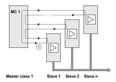
**1** Cyclic communication starts at slave 1 and ends at slave n, the cycle restarts at slave 1.
