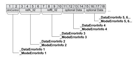
The error message is reset when the next valid data frame is transmitted.
